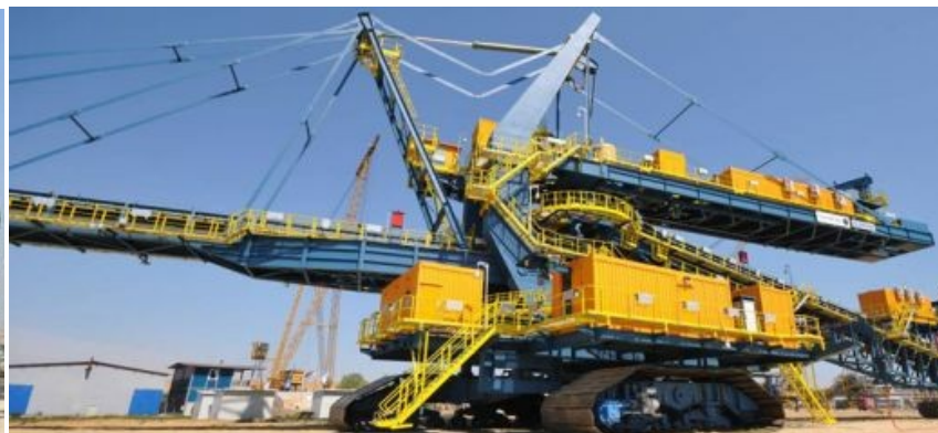
Production and assembly of spreader ARS 2000 with tripper car, TKF - Kostolac, Serbia
